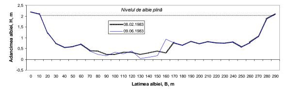
Fig. 4 Shape of the cross section of Moldova river channel in Tupilați gauging station (data source: S.M. Piatra Neamț)
